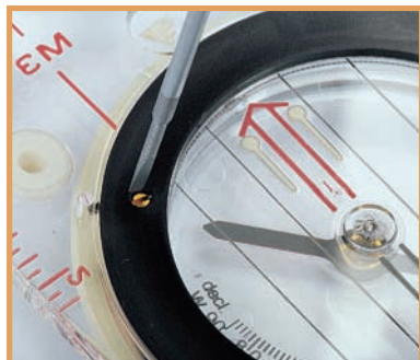
Adjusting a compass for declination
